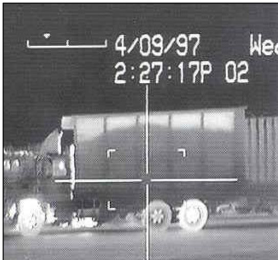
Figure 6: IRISystem Detecting Inoperable Brakes on the Vehicle (3)
